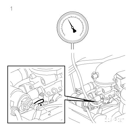
2. Connect the pressure measuring equipment to the intake manifold.
